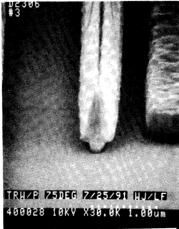
Fig. 6 a) The 0.2 \mu\text{m} InGaAs/GaAs HEMT layer structure, and b) the scanning electron microscope photograph of the 0.2 \mu\text{m} T-shaped gate.
